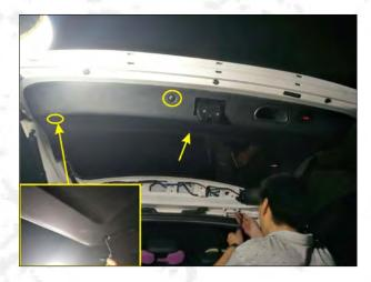
1.Remove the screws on both sides of the tailgate before removing the black cover.
