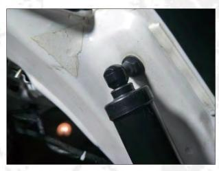
4.Install our brace rod with the original car's ball head (Same as the left and right steps).
