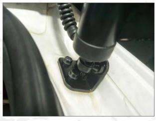
5.Remove the right and left brackets of the original car. Install the right lower bracket and brace rod, then fix them with the original car screws.
