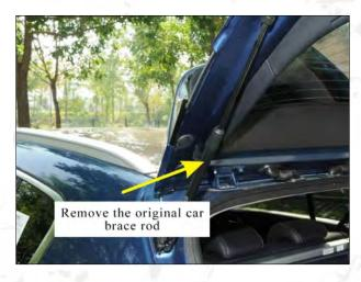
2.Remove the original car brace rod.
