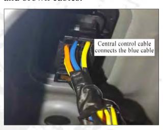
8.Lead routing. Pass the wire from the tailgate reserved hole until the door lock position. As shown in the figure.
