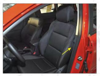
12. Find the central control cable at the position of the main driving seat B-pillar.
