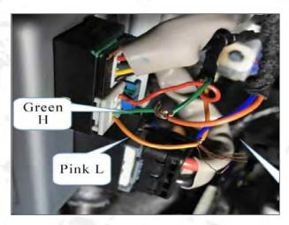
11.In the main driving, find the H and L cable connected to the white and brown cables.
