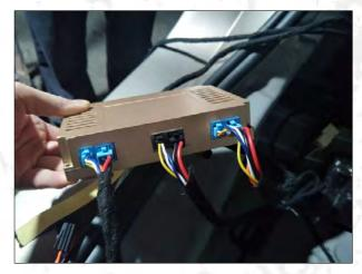
17. According to color, insert the Hall line socket, power cable socket and the electric suction lock cable socket into the control box.
