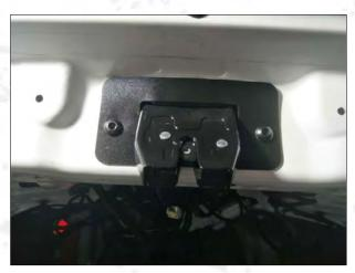
15.Remove the original car door lock. Install our electric suction lock and fix it with the original car screws.
