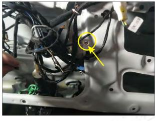
19.Install our central control box and fix it with our screws and gaskets.
