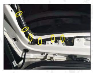
14. Power cables and central control cables are routed along the yellow line.
