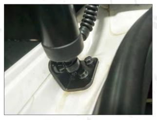
3.Remove the left lower bracket of the original car. Install the left lower bracket and brace rod, then fix them with the original car screws.
