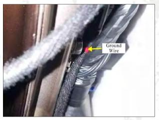
10. Connect the ground wire under the passenger seat, as shown in the figure.
