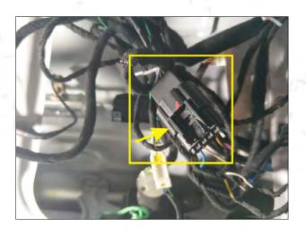
16. Connect the original vehicle unlocking plug with our three-way adapter socket. And insert the other end of the plug into the door lock position.
