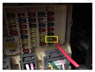
9. Ubplug the original car 20A fuse under the main driver and plug it into our power outlet.
